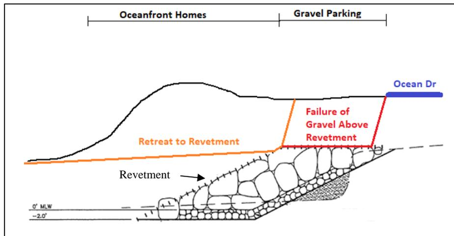
**Figure 24. General illustration of Modified Erosion Method, exposing the crest of buried revetment**
