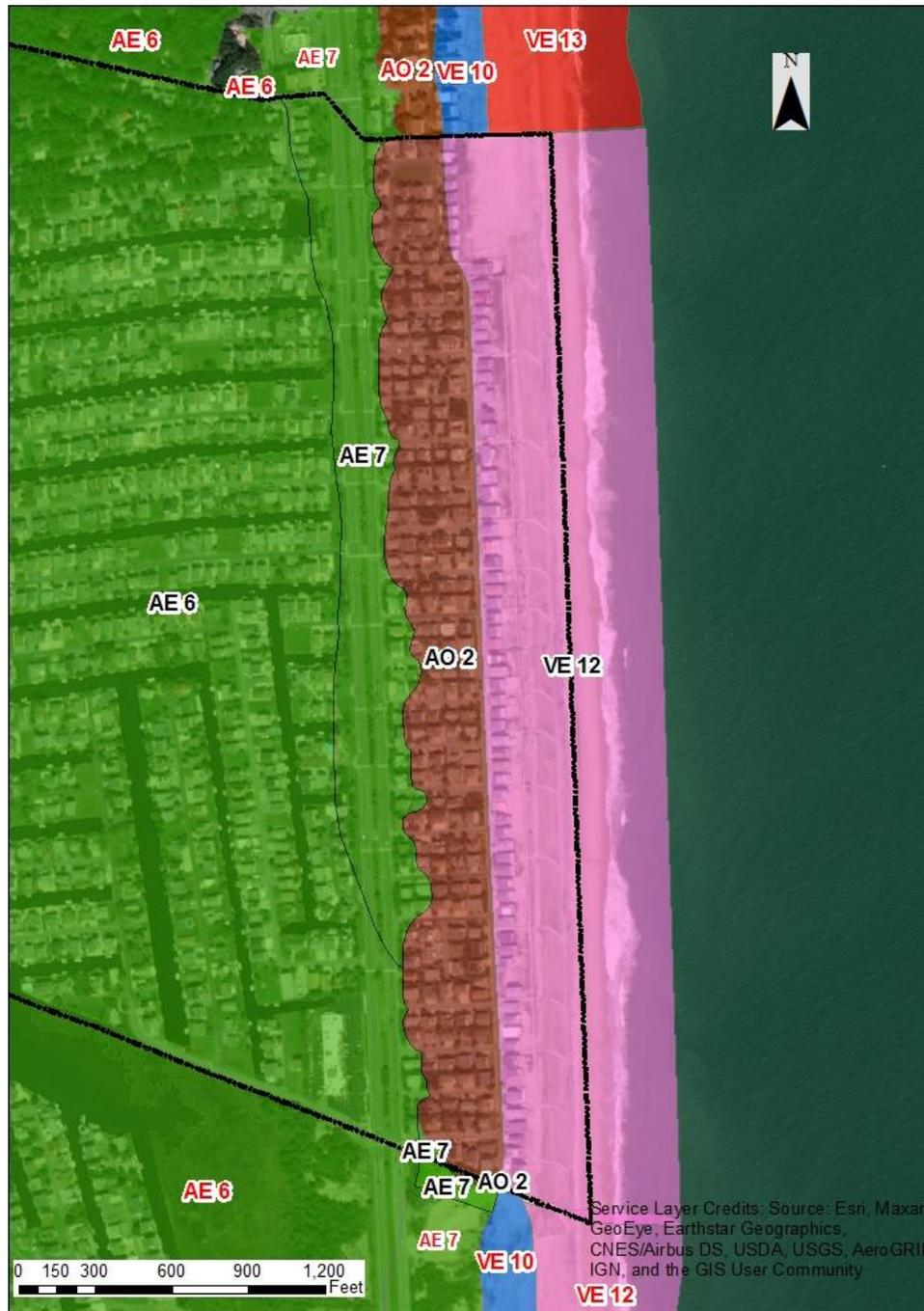
Figure 29A. Proposed mapping within Town of South Bethany (zones labeled in black) with effective mapping of surrounding areas (zones labeled in red)
