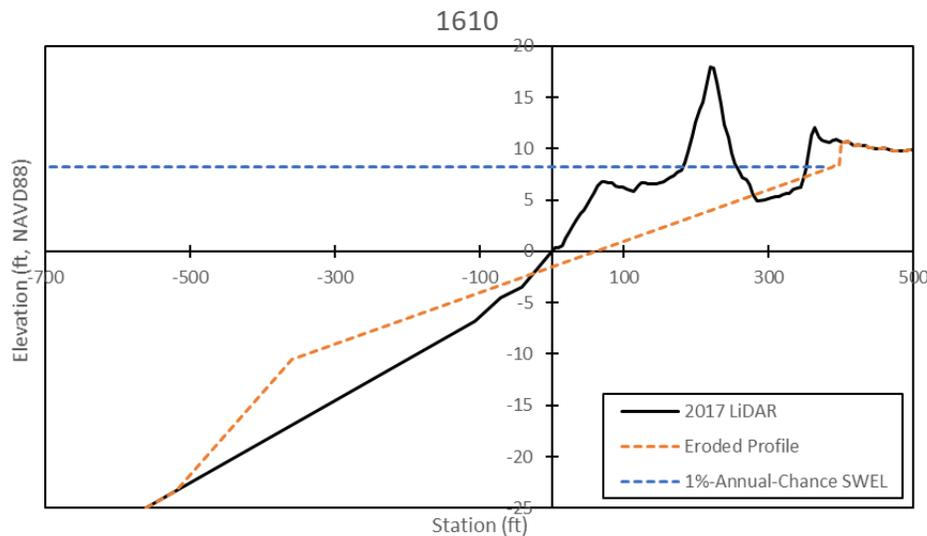
Figure 25. Example of Modified Erosion Method
