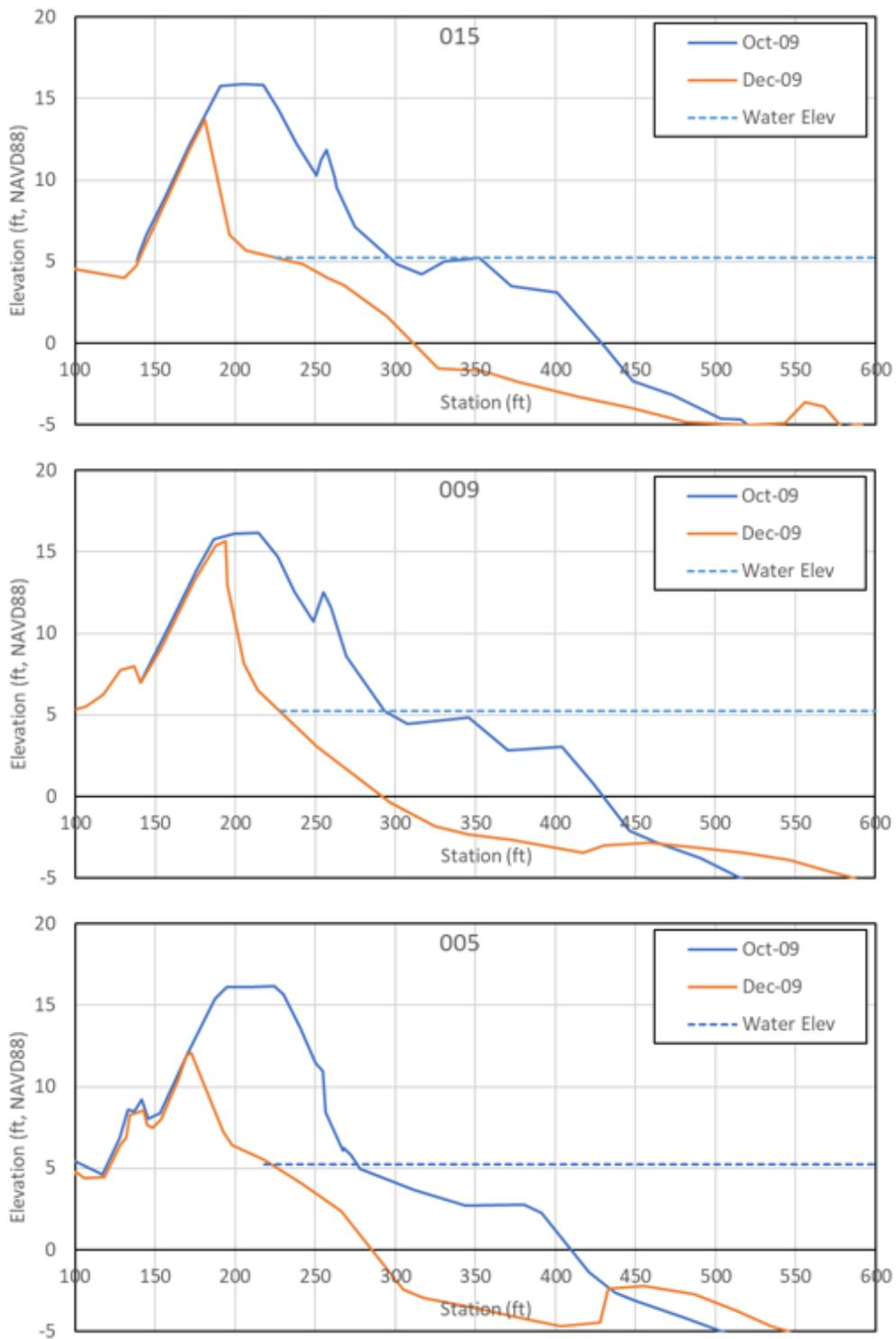
Figure 16. Nor'Ida pre- and post-storm profiles
