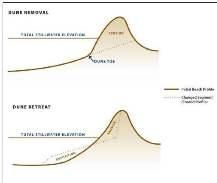
Figure 21. 540 Rule dune retreat and dune removal geometry (FEMA, 2018a)
