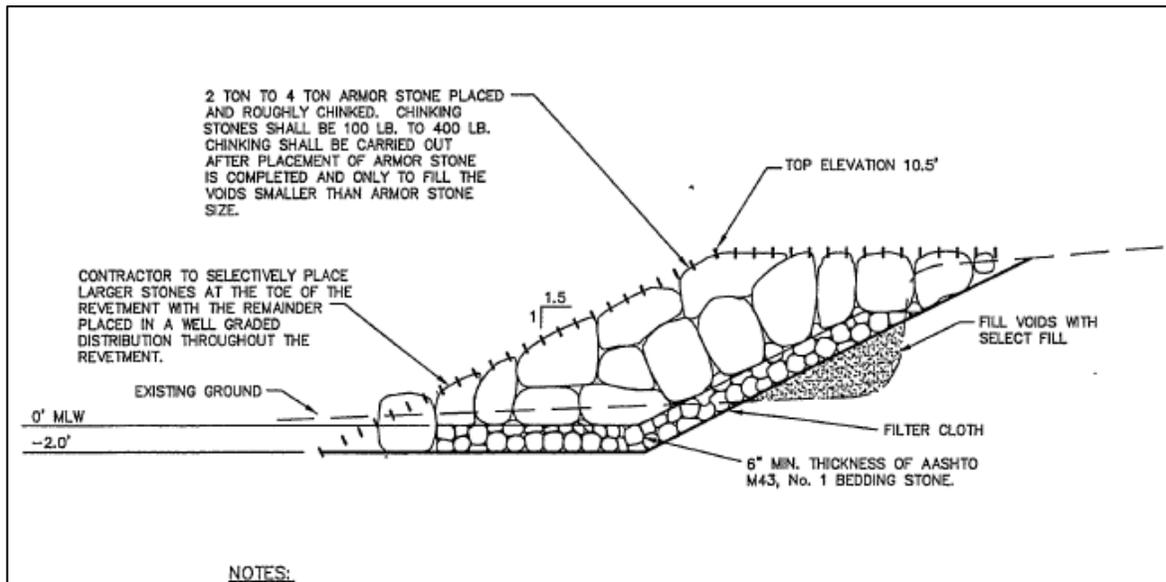
Figure 14. Revetment design specifications provided by DNREC (Soulé & Associates, 1999)
