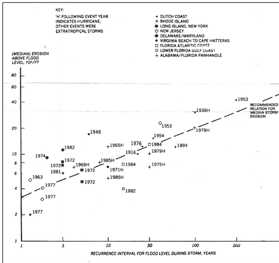
Figure 22. Median profile erosion versus recurrence interval (Dewberry and Davis, 1986)
