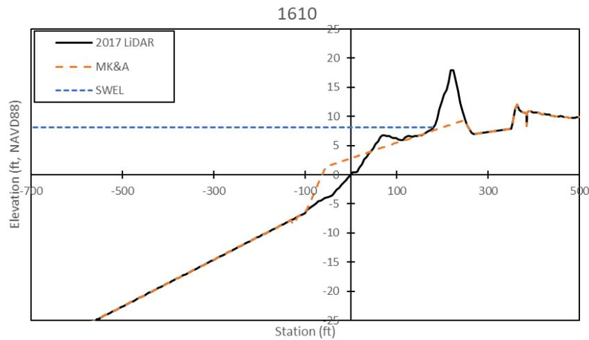
Figure 27. MK&A eroded profile for Transect 1610
