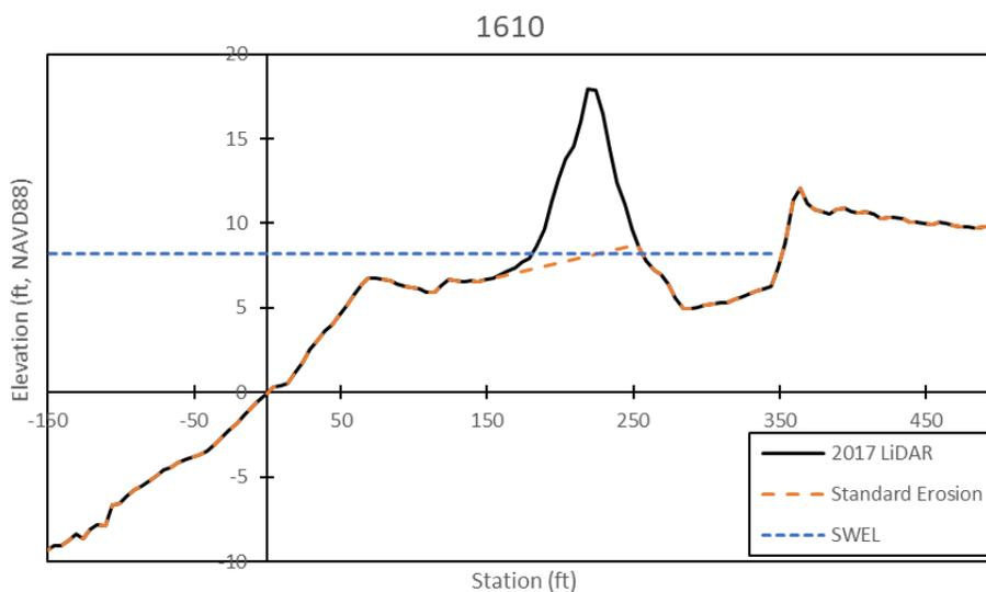
**Figure 23. Standard removal erosion geometry example for Transect 1610**
