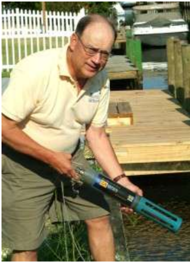
George Junkin with the Town of South Bethany deploys a continuously operating dissolved oxygen meter (YSI 6920V2) in the Anchorage Canal. Donated to the Anchorage Canal Study by the CIB.
