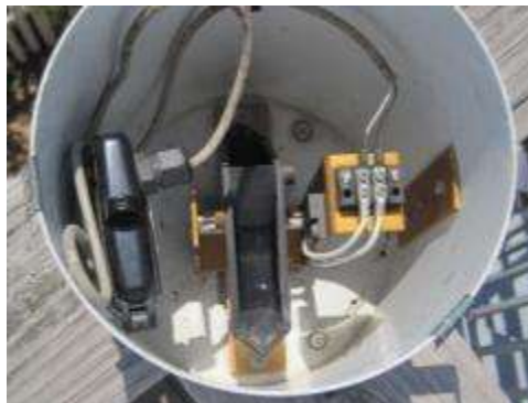
ONSET #RG2 Data Logging Tipping-Bucket Rain Gage Donated to South Bethany by DeIDOT
