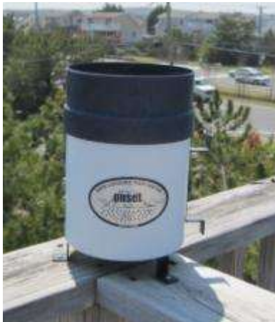
ONSET #RG2 Data Logging Tipping-Bucket Rain Gage Donated to South Bethany by DeIDOT
