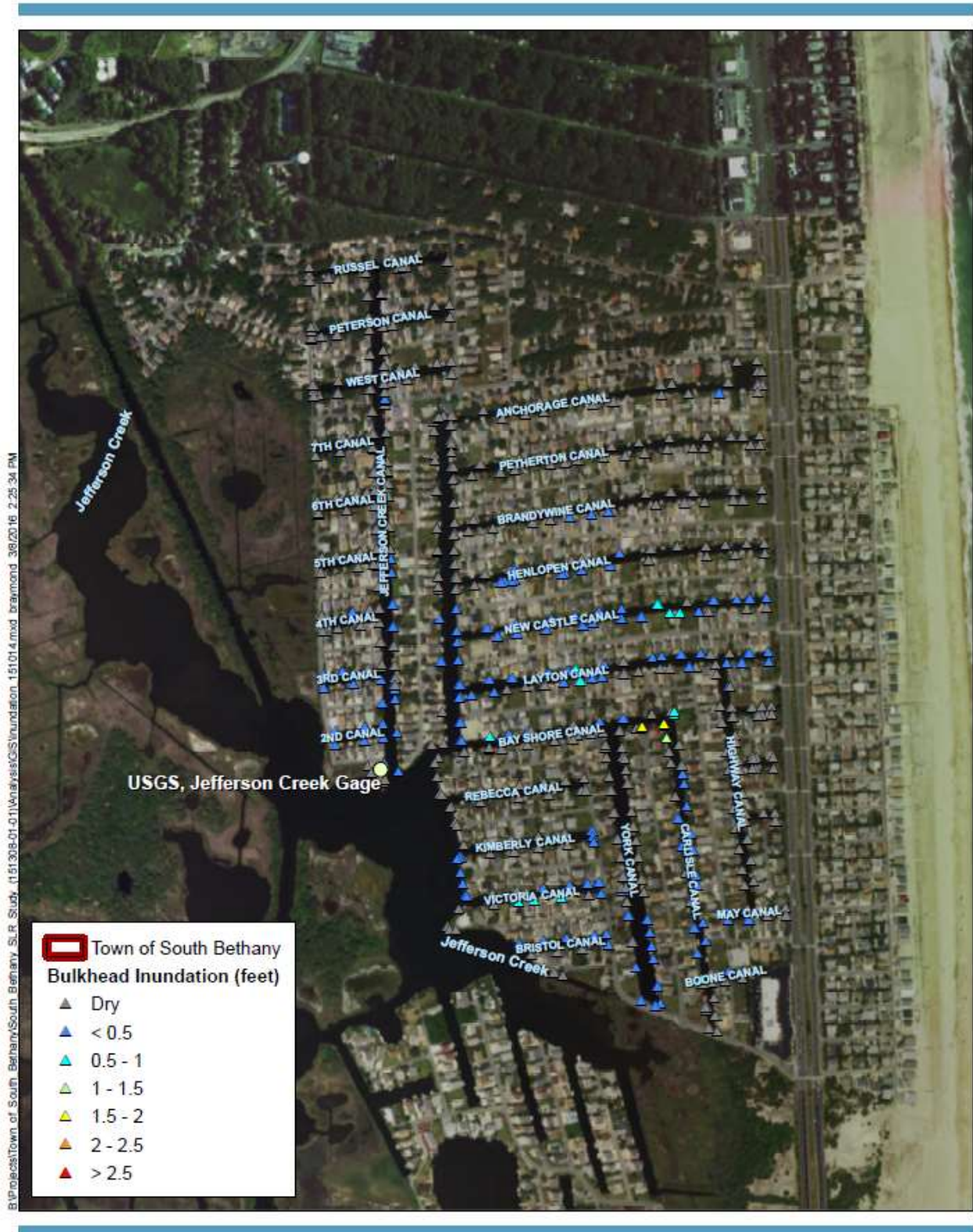
Figure 2 Bulkhead Projected 2065 Inundation Levels for Upper Bound Mean Higher High Water Level of 2.03 feet NAVD 88
