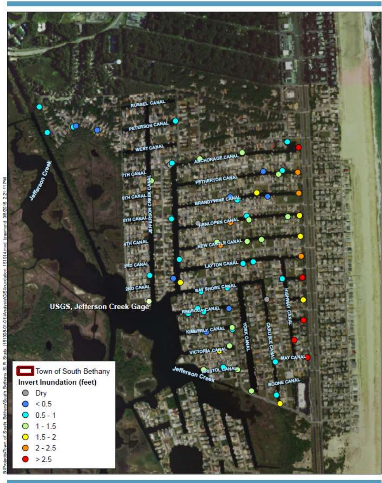
Figure 3 Outfall Invert Projected 2065 Inundation Levels for Lower Bound Mean Higher High Water Level of 1.03 feet NAVD 88
