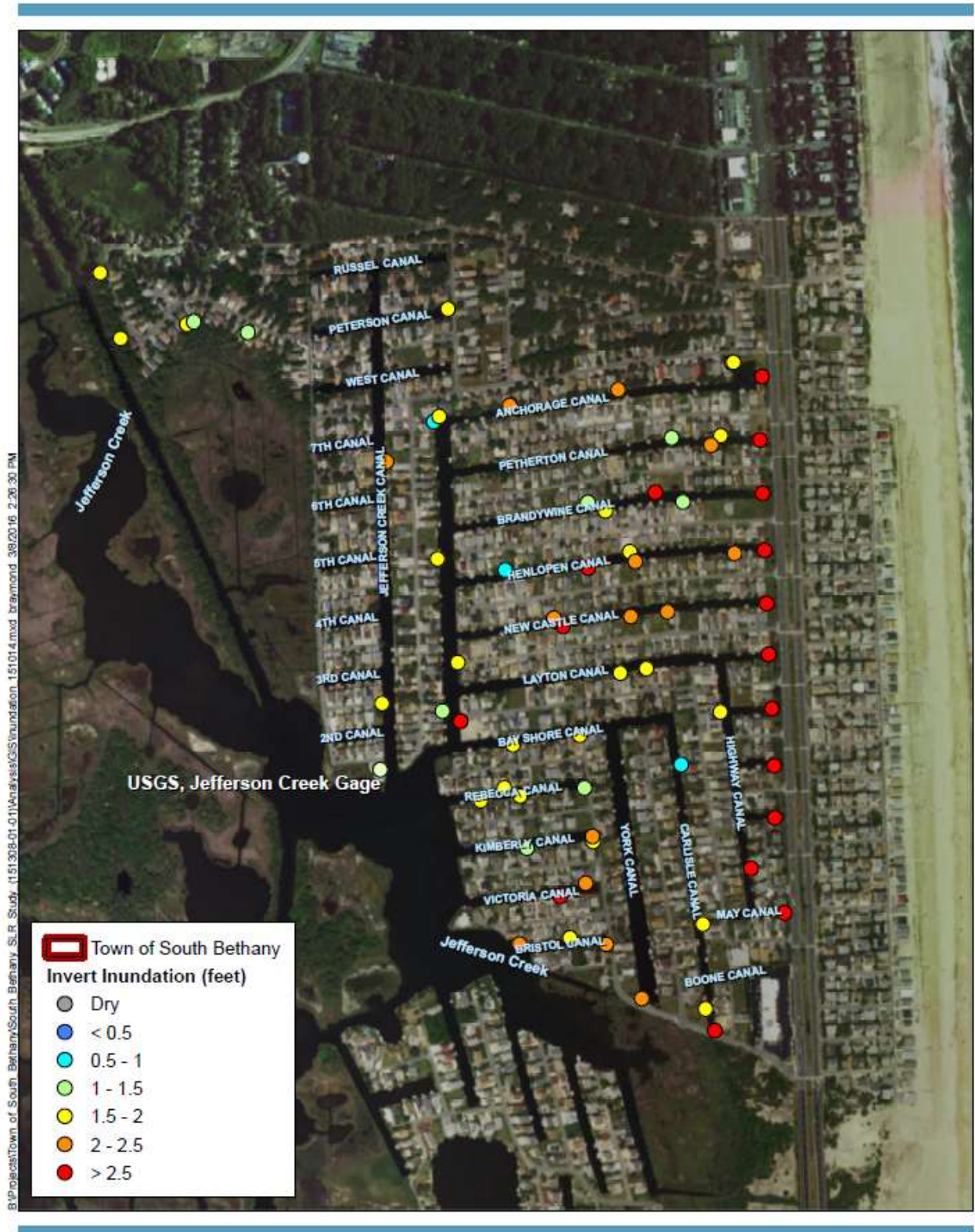
Figure 4 Outfall Invert Projected 2065 Inundation Levels for Upper Bound Mean Higher High Water Level of 2.03 feet NAVD 88
